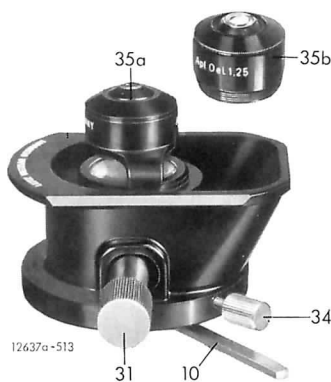
Fig. 10 Condenser bottom No 600 with the two condenser tops Ach. 0.90 and Apl. Ol 1.25. 10 Aperture iris lever 31 Rotating knob for swinging the condenser top in and out 34 Centring screws 35a Condenser top No 002 35b Condenser top No 003
