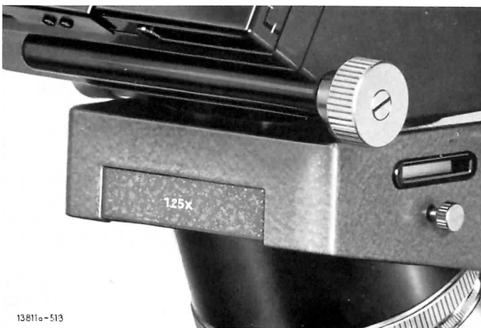
Fig. 12 Revolving nosepiece with tube factor engraved
