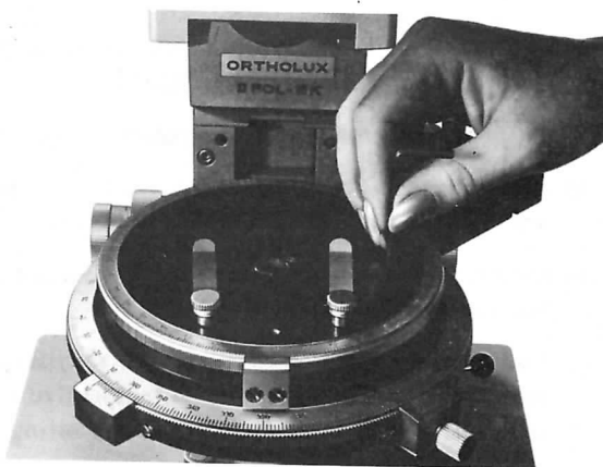
Fig. 5 Attaching the auxiliary stage
