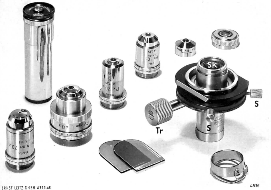
The illustration shows the phase contrast equipment with a selection of Pv objectives.
