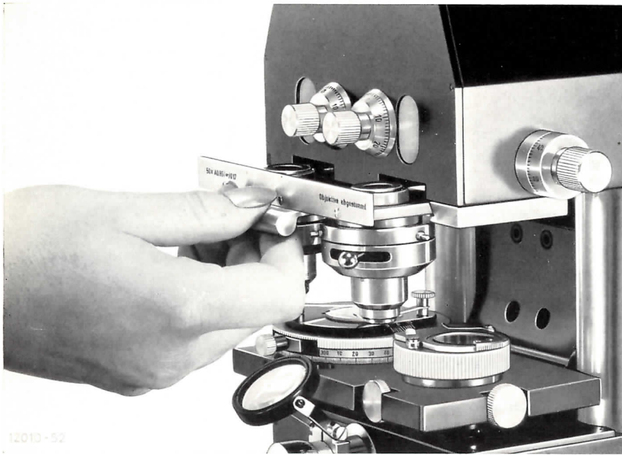
Fig. 6 Interchange of the objectives in the interference microscope.
