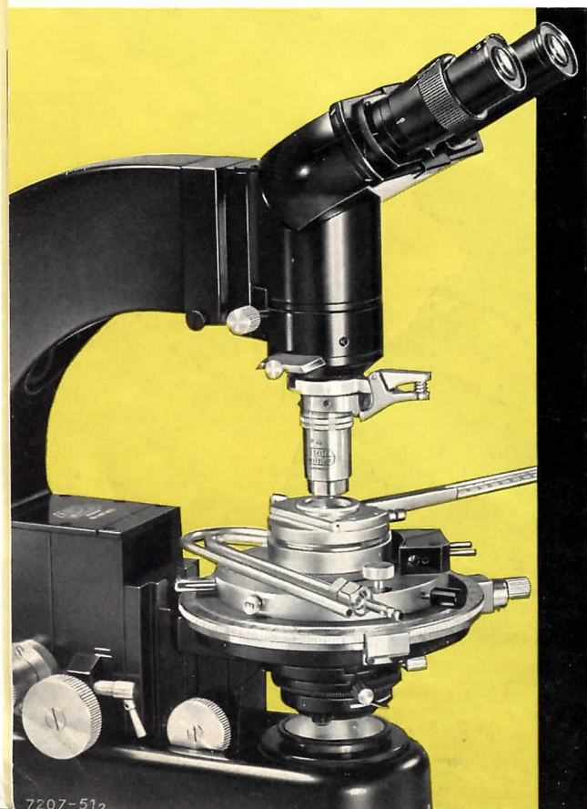
Wall and bench projection with the ORTHOLUX (above). Heating and cooling stage "350" on the ORTHOLUX (below). For the sake of clarity, the connections for heating and cooling have been omitted in this illustration.
