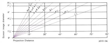
From the above table the diameter of the projected image can be seen in relation to the screen distance and the eyepiece magnification. If the screen distance and the desired diameter of the screen image are known, the necessary projection eyepiece can be determined by means of this table.
