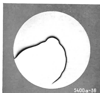
Fig. 27 Experiment showing the difference in surface tension between water and alcohol.
