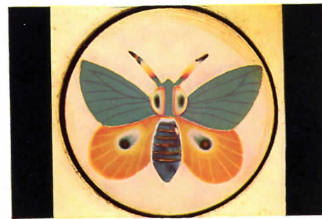
Fig. 50 Picture engraved on a small tabular crystal of gypsum seen by linearly polarized light. (a) Between crossed polarizers. (b) Between parallel polarizers.
