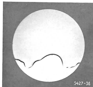
Fig. 27 Experiment showing the difference in surface tension between water and alcohol.
