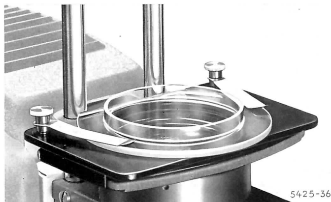
Fig. 25 Method of mounting a glass dish on the vertical projection attachment, for showing phenomena occurring at the liquid surface.
