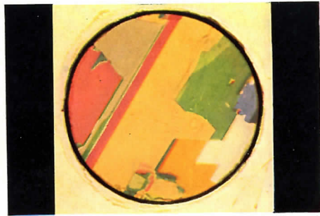
Fig. 49 Mica in linearly polarized light. (a) Between crossed polarizers. (b) Between parallel polarizers.
