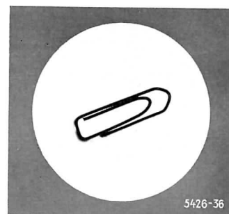
Fig. 26 Paper clip kept floating on water by surface tension.
